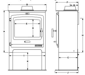
A 588mm C 260mm E 350mm G 112mm I 500mm K 250mm B 524mm D 254mm F 310mm H 451mm J 330mm
