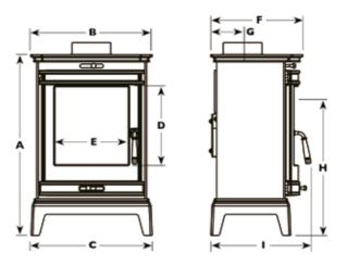
A 637mm C 427mm E 260mm G II3mm I 353mm B 430mm D 275mm F 326mm H 507mm
