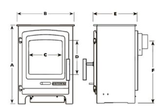
A 568mm C 260mm E 305mm B 413mm D 237mm F 450mm
