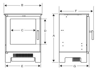
A 582mm C 288mm E 400mm G 337mm B 430mm D 304mm F 389mm
