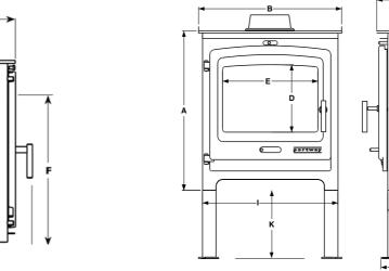
A 588mm C 260mm E 350mm G 112mm I 500mm B 524mm D 254mm F 310mm H 451mm J 310mm K 150/300mm High/Low Legs
