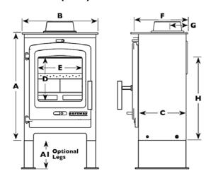
A 588mm C 260mm E 247mm G 112mm B 414mm D 249mm F 295mm H 451mm AI 150/300mm
