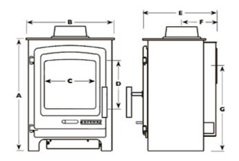
A 573mm C 260mm E 346mm G 463mm **B 413mm D 237mm F 163mm** (138mm using optional flue casting collar)
