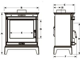
A 637mm C 326mm E 360mm G 113mm B 532mm D 275mm F 352mm H 506mm
