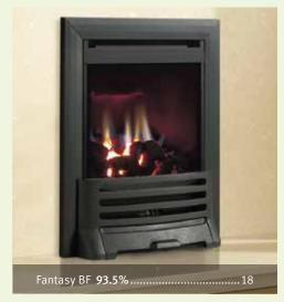
Our range of high efficiency balanced flue fires have an energy efficiency of up to 93.5%. Designed for those who want all the benefits of a gas fire but don't have a built in chimney or flue in their home, a balanced flue fire comes with its own flue terminal which is vented directly through an outside wall. They are glass fronted, completely room sealed appliances and work by drawing and venting external air via a pair of co-axial tubes into the fire for combustion purposes.
