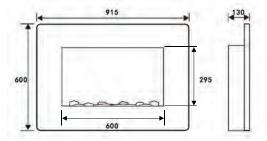
Please note: When installed there must be a minimum distance of 400mm between the bottom of the fire and the floor.
