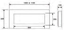
Please note: When installed there must be a minimum distance of 400mm between the bottom of the fire and the floor.
