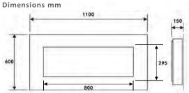
Please note: When installed there must be a minimum distance of 400mm between the bottom of the fire and the floor.
